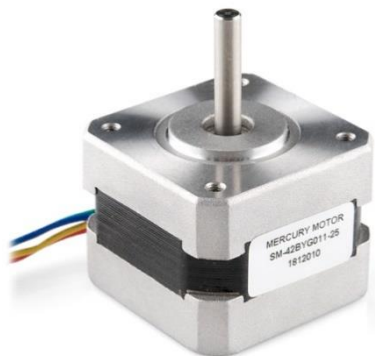
Figure 3: A bipolar stepper motor with permission from Sparkfun Electronics
